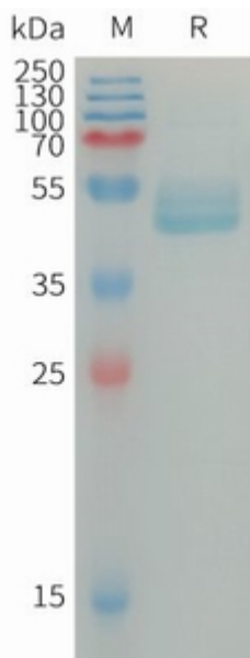
Figure 1. Human IL4 Protein, mFc Tag on SDS-PAGE under reducing condition.
