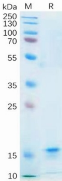
Figure 1. Human IL21 Protein, His Tag on SDS-PAGE under reducing condition.
