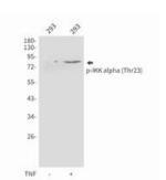
Western blot analysis of Phospho-IKK alpha (Thr23) in 293 lysates using Phospho-IKK alpha (Thr23) antibody.
