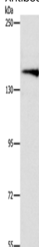
Gel: 6% SDS-PAGE, Lysate: 40 µg; Lane: Mouse brain tissue; Primary antibody: 220312 (ARHGEF11 Antibody) at dilution 1/1000; Secondary antibody: Goat anti rabbit IgG at 1/8000 dilution; Exposure time: 1 minute
